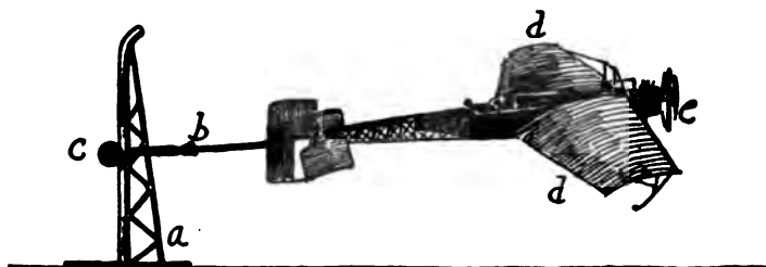
FIGURE 169.—Bleriot Starting Device. The aeroplane is hooked by the rope b to the pulley c , which runs along the rear edge of the pillar a . By starting the propeller the back draft of air thrown under the wings d is expected to lift the machine until c runs off the top of a .
