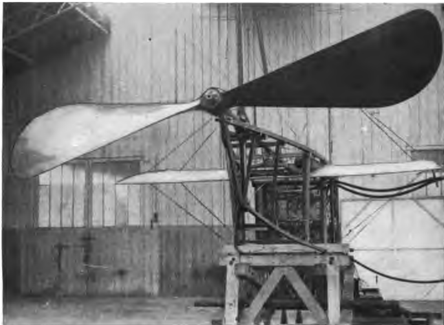
FIGURE 103.—Wooden Propeller Applied to Car of Clement Dirigible Balloon.
