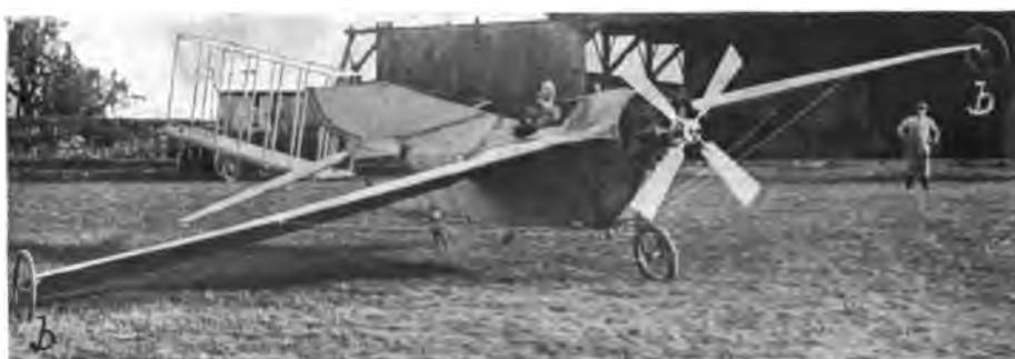
FIGURE 223.—Three-Quarters View of the R. E. P. Monoplane. The wing wheels b b and the twisting rudder h are features of this machine.
