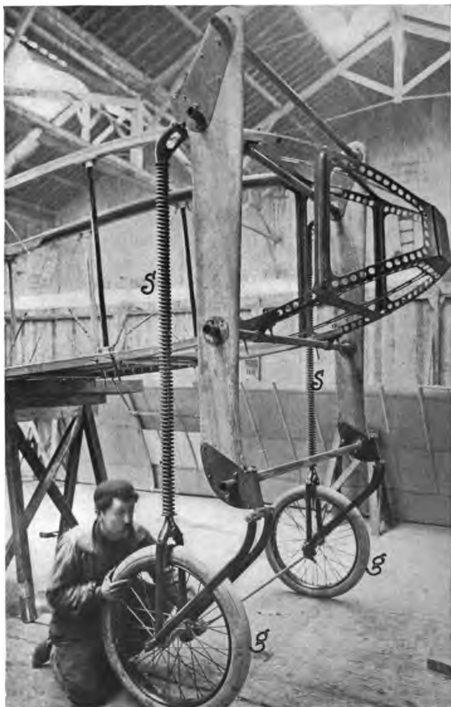
FIGURE 170.—Typical Allighting Gear. In this the upward swing of the wheels u y on their link connections is cushioned by the helical springs s s' .
