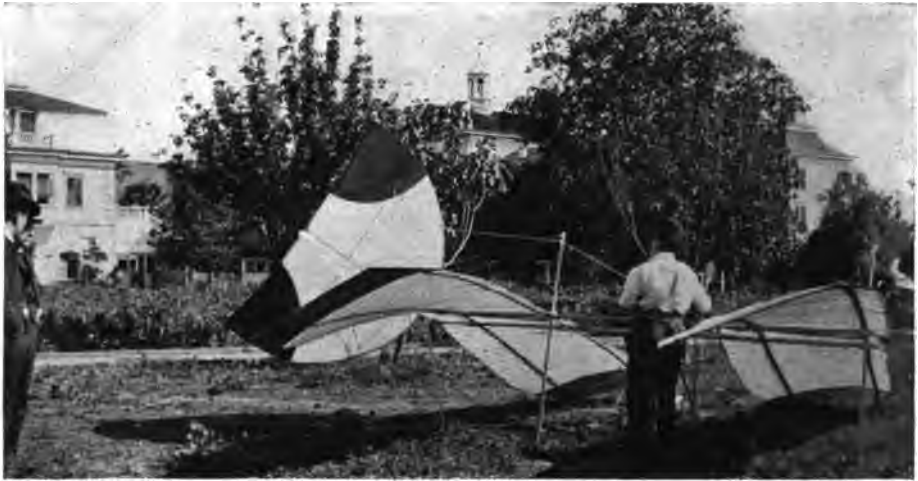
FIGURE 226.—Side View of Montgomery Double Monoplane Glider. This machine was probably built on more scientific principles than any other so far constructed. On at least three occasions operators have deliberately turned side somersaults with it, besides which many descents have been safely made from heights ranging up to 4,000 feet, at speeds said to have ranged as high as 68 miles an hour. Its equilibrium is so positive that it automatically rights itself when released upside down in the air.
