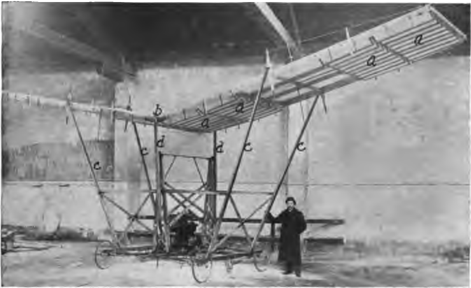
FIGURE 27. —Collomb Ornithopter. This machine is of the direct, orthogonal flapping-wing type, provided with valvular flaps at a a a a . The two wings, which pivot at the upper extremities of the links c c c c , are reciprocated by the vertical reciprocation of the arms d d .
