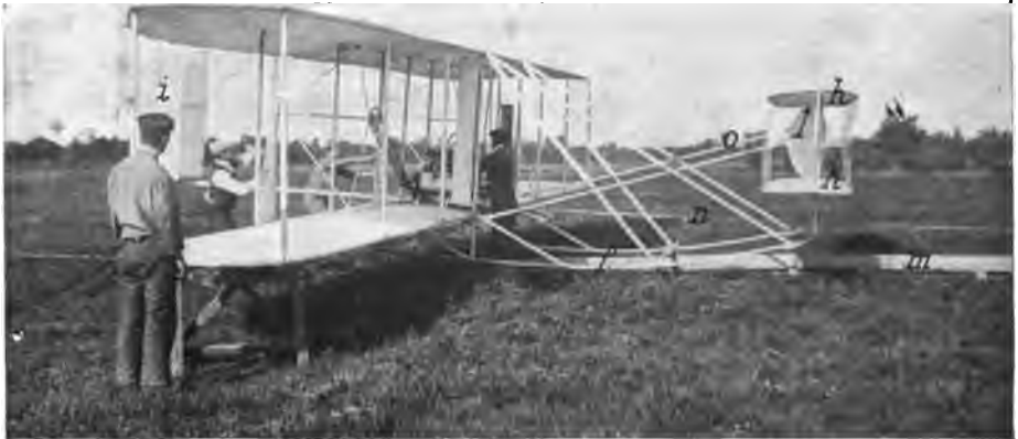
FIGURE 163.—Wright Machine on Starting Rail. The starting rail is at m , n is the connection of the rope by which the starting impulse is given, f are the runners, h is the elevator, o is the elevator control rod, i is the rudder, and l is one of the steadying planes peculiar to this machine.
