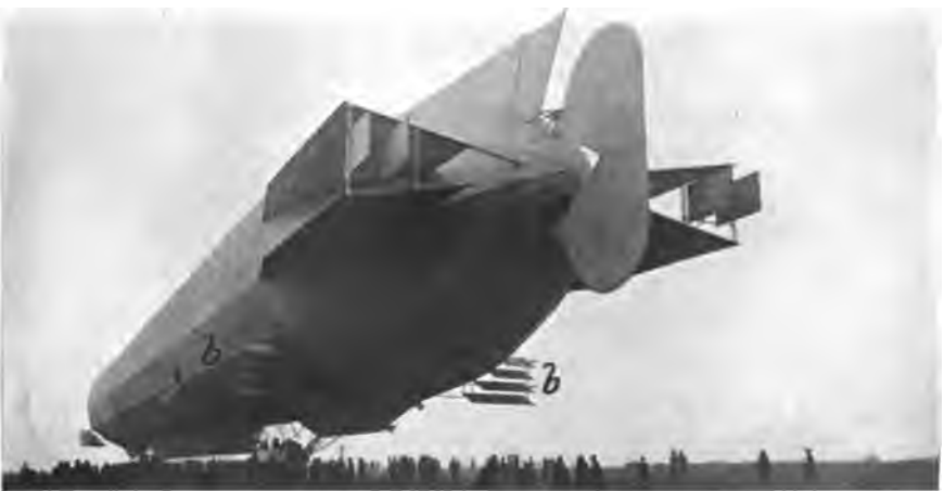
FIGURE 17.—The latest Zeppelin Dirigible. The upper picture shows the rigid construction very clearly, while in the different views the stabilizing fins c , the dipping planes bb , and the rear rudder a , are clearly shown.
