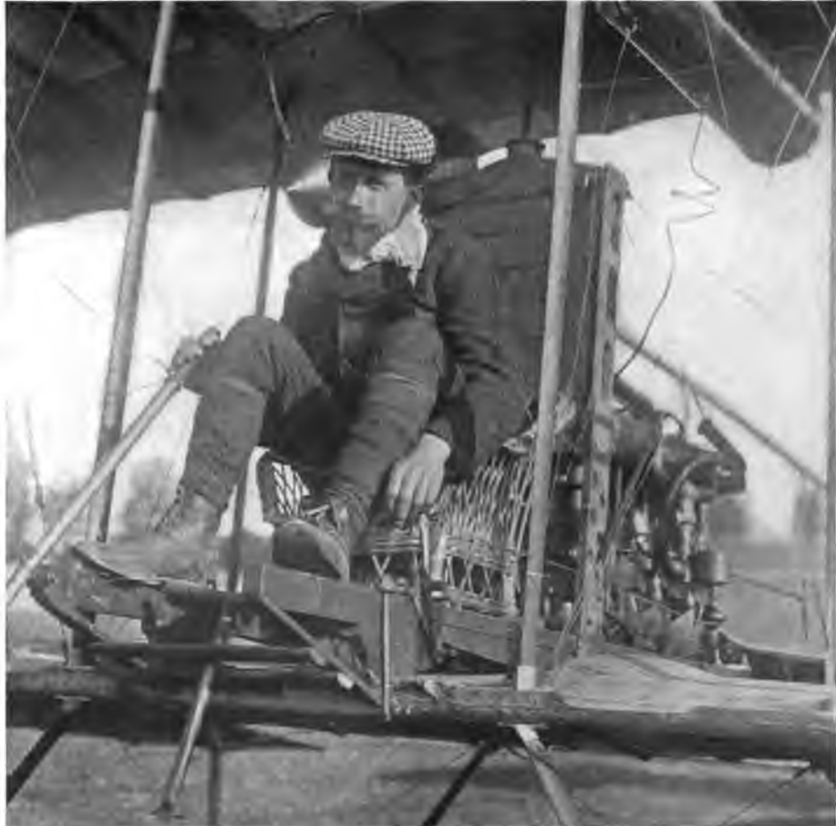
FIGURE 248.—Wicker Chair and Foot Control of Allerons in Sommer's Farman Biplane.
