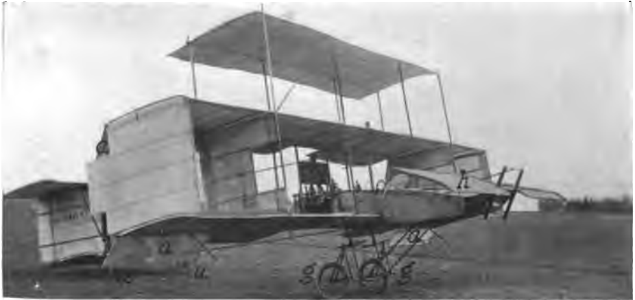
FIGURE 211.—Farman's Modified Voisin. Note the ailerons at a a , and the added upper surface, making the machine a triplane.
