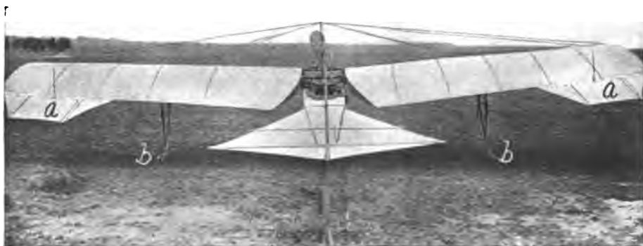
FIGURE 214.—Rear View of Antoinette V. In this view the allerons a a and the balancing rollers b b are well shown.
