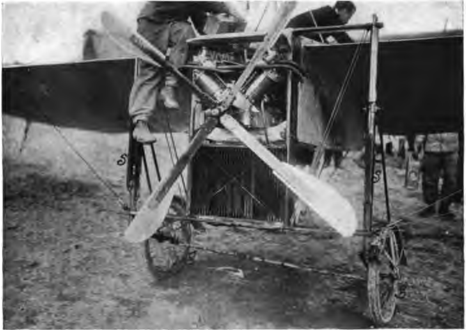
FIGURE 171.—Details of Bleriot Monoplane. This is one of the earlier machines of the "Bleriot XI" type, and is provided with an eight-cylinder, water-cooled motor, with radiator immediately beneath it. The wheels g g and the rubber springs s s are characteristic of the Bleriot alighting gear, but in the case of the latter the multiplication of the movement as shown in this view by passing over rollers has been abandoned.
