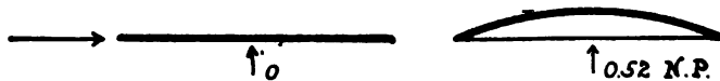
FIGURE 43.—Comparison of Plane and Arched Surfaces Without Angle of Incidence. Lilienthal found that while the lift of a flat surface placed as above was zero, the arc of a circle gave a lift equal to 52 percent of the pressure upon it when exposed in a vertical position to the same wind.
