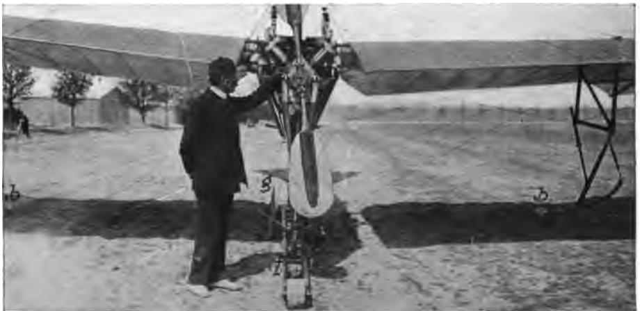
FIGURE 176.—Alighting Gear of Antoinette Monoplane. Most of the weight is carried on the two center wheels g g , with the spring-mounted spherical wooden rollers at b b to balance the machine. The runner f is an additional safeguard against shock in landing.
