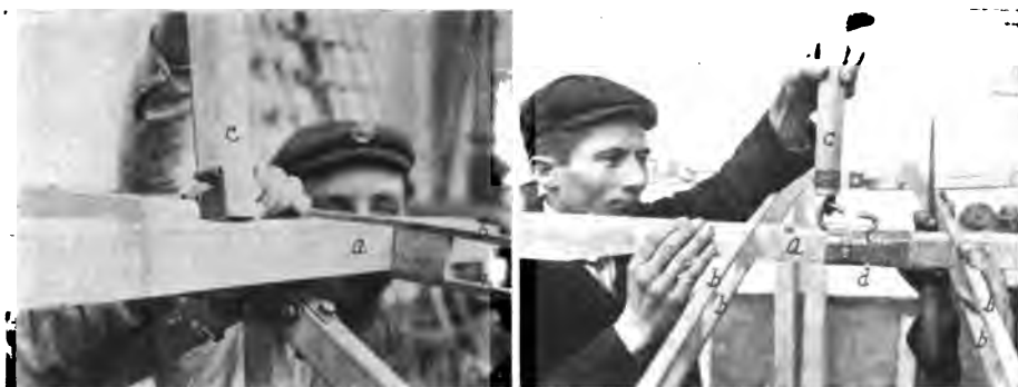
FIGURE 192.—Details of Wright Biplane Strut Connections. Note the manner in which the struts c are fastened in U-shaped metal sockets at the center of the machine and hooked to the wing bars a in the flexible wing ends. The plate d indicates the point at which the wings unship for convenience in shipping and storing, while b b are the double rib members.
