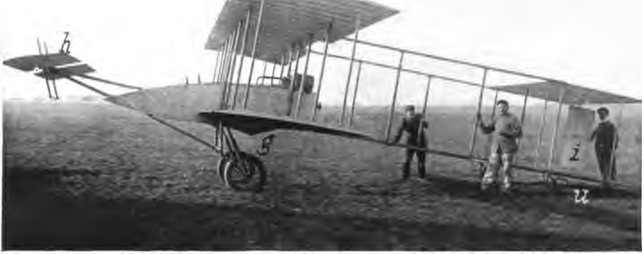
FIGURE 209.—Side View of Maurice Farman's Biplane. This machine resembles both the Voisin and the Farman machines—the former in its running gear and the latter in the absence of the vertical panels.
