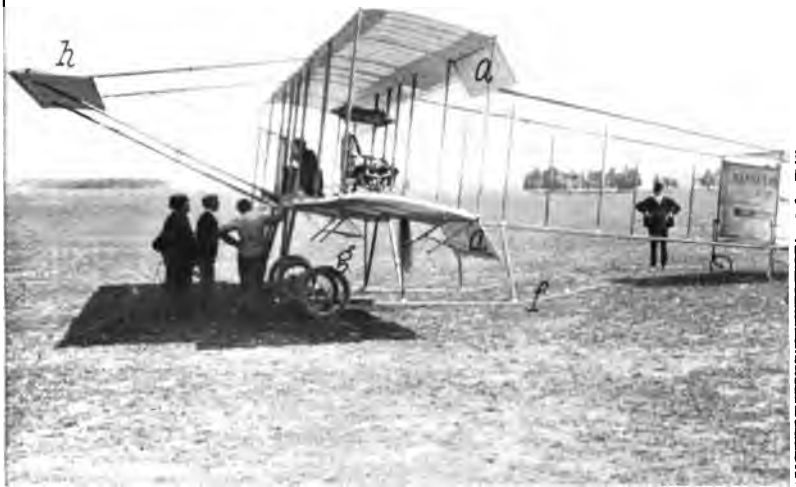
FIGURE 207.—Side View of Farman Biplane. This machine, which holds distance and duration records, is particularly interesting because of the use of the combination with the runners f in the alighting gear.
