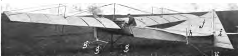
FIGURE 216.—Rear View of Antoinette VII. This is the machine with which Latham flew 20 miles in his second attempt to cross the English Channel. Allerons are discarded in favor of rocking the whole wing, and the alighting gear is reduced to the wheels g g g and u .
