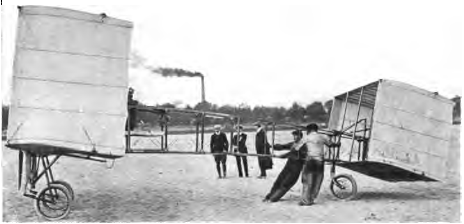
FIGURE 203.—Latest Model Voisin Biplane.—With tractor screw and no front elevator.
