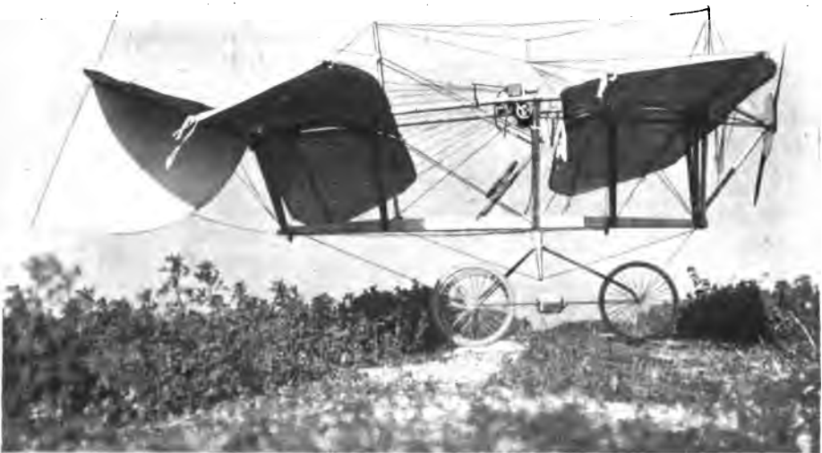
FIGURE 227.—Side View of Small, Power-Propelled Montgomery Double Monoplane. This machine has a wing spread of 26 feet, an area of 250 square feet, and weighs from 400 to 450 pounds, including the weight of the operator and the fuel. It flies at a speed of over 30 miles an hour with less than six horsepower, and employs more deeply cambered curves than have been successfully used in any other machine. Its stability is inherent in the form of its surfaces rather than dependent upon the manipulation of balancing devices, so that if dropped upside down it will invariably right itself and commence gliding with a fall of not over four or five times the span of its wings. The large vertical surface at the rear has no movement sidewise, being a stabilizing fin, not a rudder.
