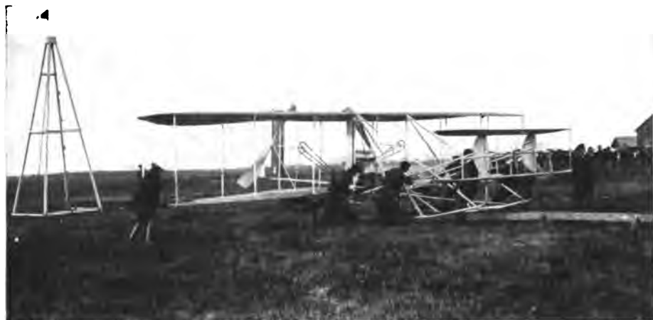
FIGURE 166.—Wright Machine on Starting Rail, with Starting Derrick in the Background
