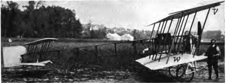
FIGURE 60.—Goupy Biplane. In this the placing of the surface v in advance of the surface w is intended to cause the air-currents to meet the surfaces in such a manner as to secure greater lift from the upper surface than is secured in biplanes in which it is placed farther back. That flatness of the surfaces is quite erroneous, though perhaps not the only reason the machine failed as a flier.
