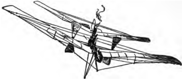
FIGURE 70. —Langley's 25-Pound Double Monoplane, With Wings at Dihedral Angle. This model on May 6, 1896, flew for more than half a mile over the Potomac River, at a speed of about 20 miles an hour. Subsequently, on November 28, 1906, with a similar model weighing about 30 pounds, a three-quarter mile flight at about 30 miles an hour was achieved. This was at the end of a three years' period of experimenting that had for its object the ultimate production of a man-carrying machine. The size of the heavier model was a little over 12 feet from tip to tip, with a length of about 16 feet. The whole power plant, which consisted of a 5-pound boiler and a 26-ounce non-condensing steam engine that developed 1\frac{1}{2} horsepower, weighed about 7 pounds. Propulsion was by bevel-gear driven, two-bladed twin screws, rotating in opposite directions behind the forward surfaces at about 1,200 revolutions a minute. The hull was metal sheathed to protect the burner from the wind, and the vessel between the forward surfaces was a float to keep the machine up when it alighted upon the water. In conjunction with the experiments with a man-carrying machine, which terminated with the unsuccessful launching on December 8, 1903, a model similar to the above, but weighing 58 pounds and having 66 square feet of sustaining surface—it being a one-fourth size copy of the large machine—was successfully flown with its 3-horsepower motor.
