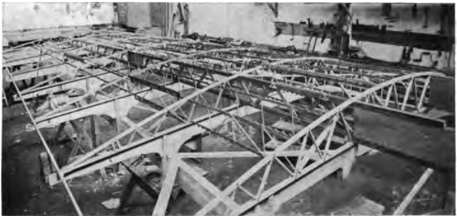
FIGURE 71.—Internal Framing of Antoinette Monoplane Wing.
