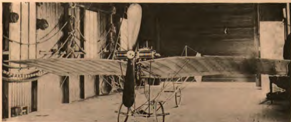
FIGURE 220.—Front View of Santos-Dumont's "Demoiselle." This machine, which weighs less and costs less than many motorcycles, is the smallest machine that has successfully flown.
