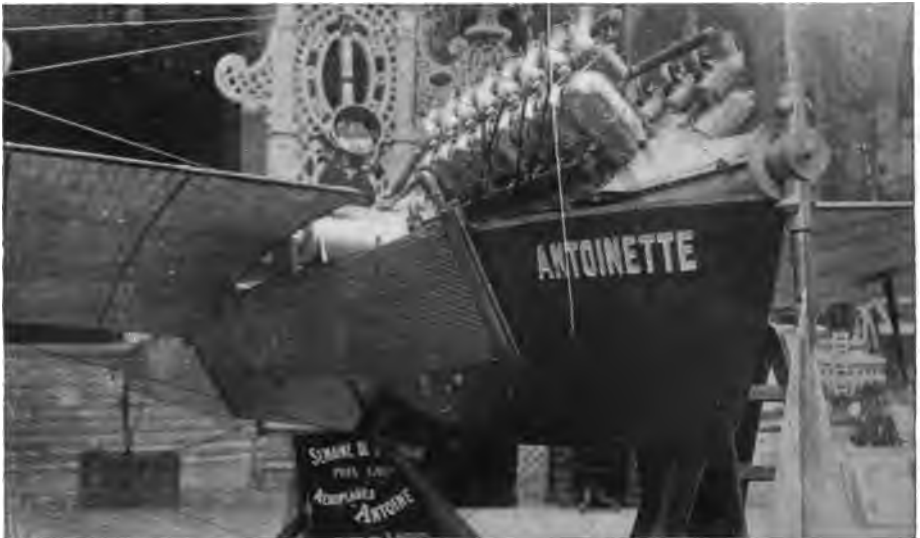
FIGURE 175.—Boat-like Body of Antoinette Monoplane. This machine, which is equipped with a hundred horsepower motor, will run on the land, in the water, and in the air.
