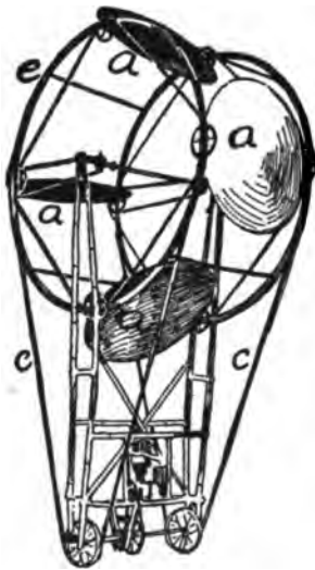
FIGURE 90. — Feathering-Paddle Flying Machine. By the rotation of e by the belt c it was expected that the paddles aaac would sustain the weight by beating down on the air, it being noted that they come down flatwise but rise edgewise through the action of the feathered mechanism.
