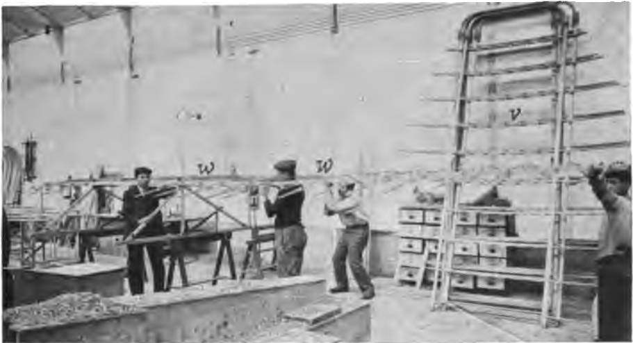
FIGURE 75. —Assembling Wright Wing Frames. The complete biplane is made in three portions, the center section slightly overhanging the two runners—between which stands the man at the left of the view. This section has attached at each end a section like that at w —shown at the moment of attachment. Similar sections are leaning against the wall at v .
