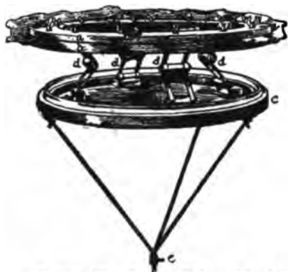
FIGURE 10.—Balloon Valve. The fabric at the top of the gas bag is clamped between the rings a b , and the opening through these rings is kept normally closed by the disk c , held in place by the pressure of the gas and the tension of the spring hinges d d d d , but a pull on the cord e serves to open the valve, permitting the escape of any desired quantity of gas.
