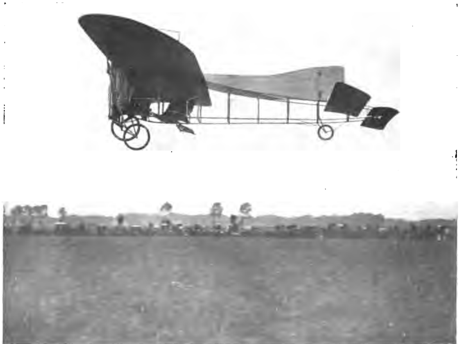
FIGURE 158. —Bleriot XII in Flight. This monoplane carries three passengers.
