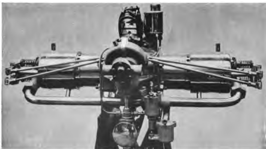
FIGURE 116.—Darracq and Duthell-Chalmers Aeronautical Motors. The Darracq—in the lower view—is the engine with which Santos-Dumont achieved his recent successful monoplane flights. It weighs 66 pounds and develops 35 horsepower. Of particular interest in the other motor is the flywheel a , with steel rim and wire spokes.
