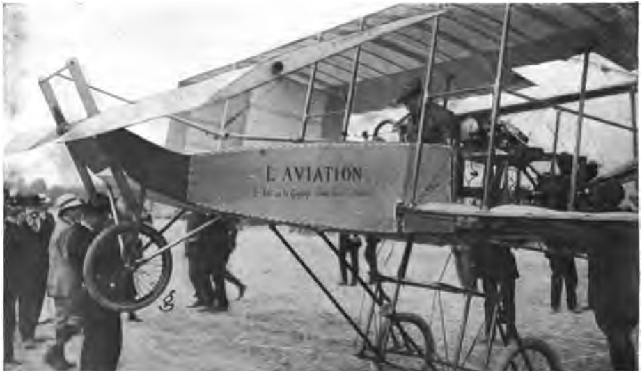
FIGURE 172.—Alighting Gear of Paulhan's Voisin. The wheel g on the prow is a safeguard against undue forward inclination of the machine in landing.
