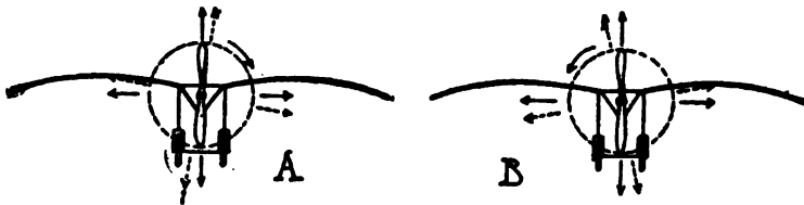
FIGURE 106.—Effect of Gyroscopic Action of a Single Propeller on Steering. With the directions of rotation shown, effort to steer in the direction of the solid arrows results in deviation in the direction of the dotted arrows, to an angular extent varying with the magnitude of the gyroscopic effect. This tendency can, of course, be allowed for by a practised operator. In both views the machine is to be regarded as approaching the observer.
