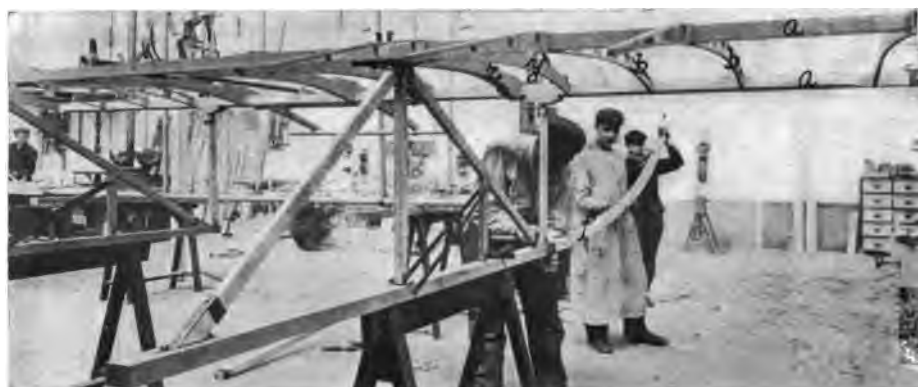
FIGURE 193.—The Wright Runner Construction. The solid ribs bb serve to support the motor, operator, etc. The other ribs bb are so built up as to enclose the wing bars aa between the double surfacing of fabric. The attachment of the forward curved members of the runners at f is clearly apparent upon close examination.
