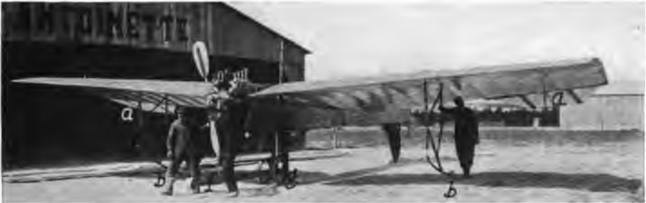
FIGURE 76. —Alleron Control of Lateral Balance in Antoinette Monoplane by manipulation of the two hinged tips aa .
