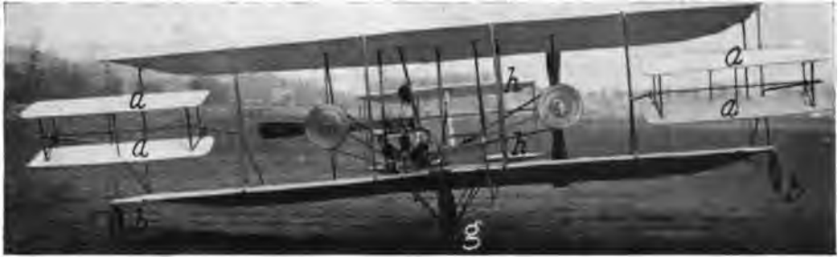
FIGURE 78.—Lejeune Biplane, with forwardly-extended allerons at aaaa , for maintaining lateral balance.
