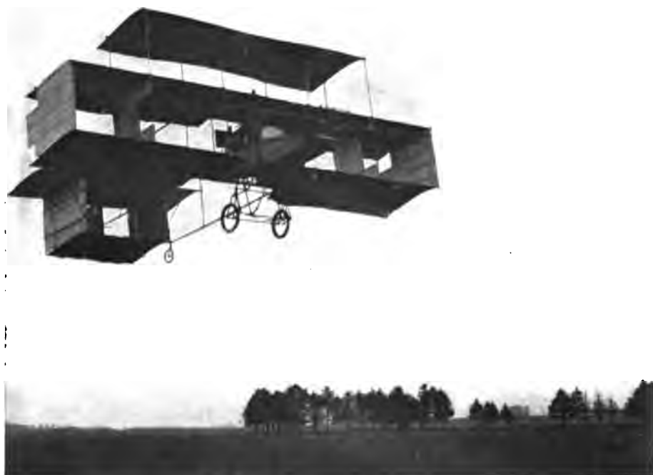
FIGURE 142.—Voisin Biplane Modified into a Triplane.
