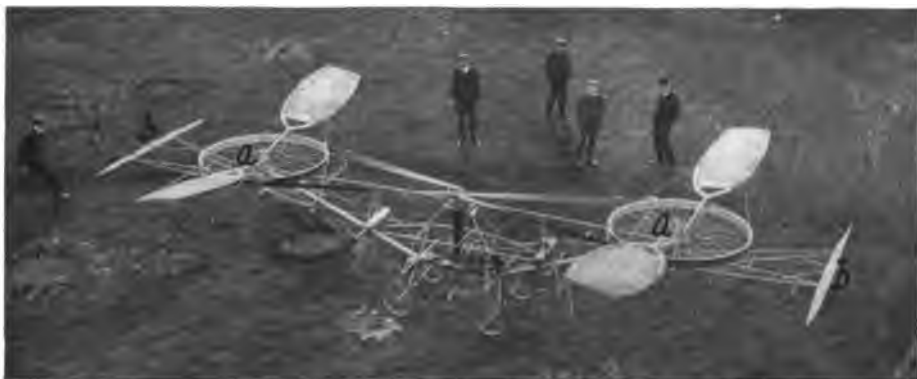
FIGURE 32.—Cornu Helicopter. This curious-appearing contrivance is the creation of a prominent European engineer who has given years of study to this problem. The two lifting propellers at aa are mounted on bicycle-like wheels and are belt-driven in opposite directions from a vertical shaft. The flat surfaces bb are for lateral control and steering.
