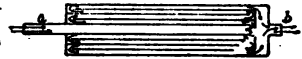
FIGURE 129.—Muffler. The gases entering at a flow back and forth as indicated by the arrows until they issue from the vent b .
