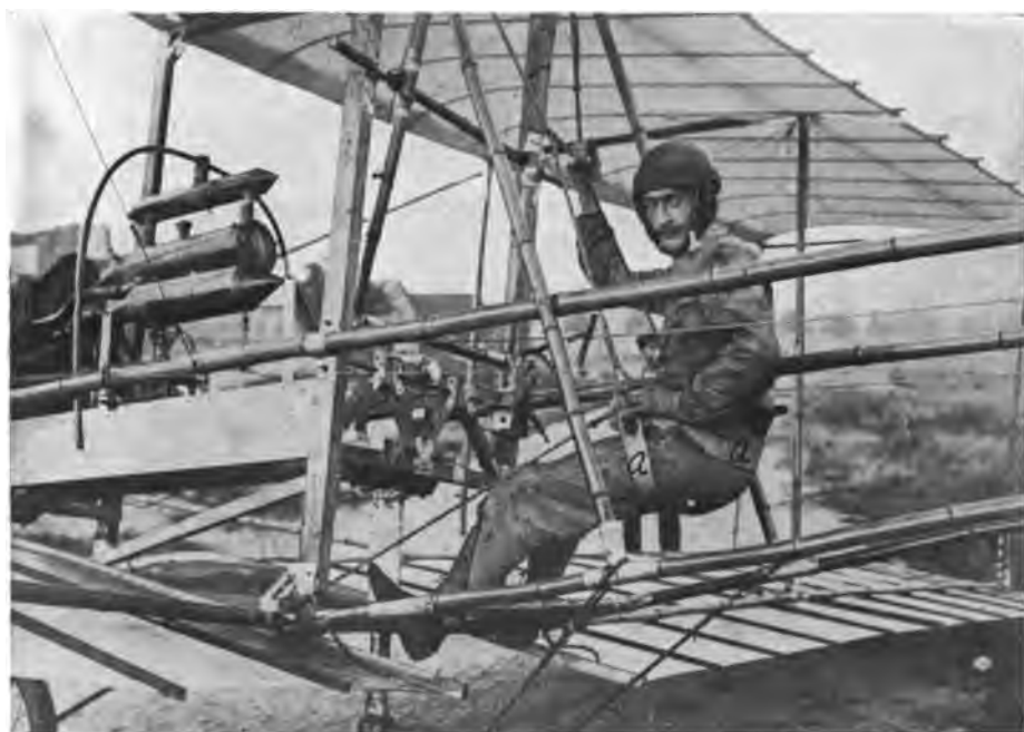
FIGURE 251.—Sling Seat of Captain Ferber's Biplane.
