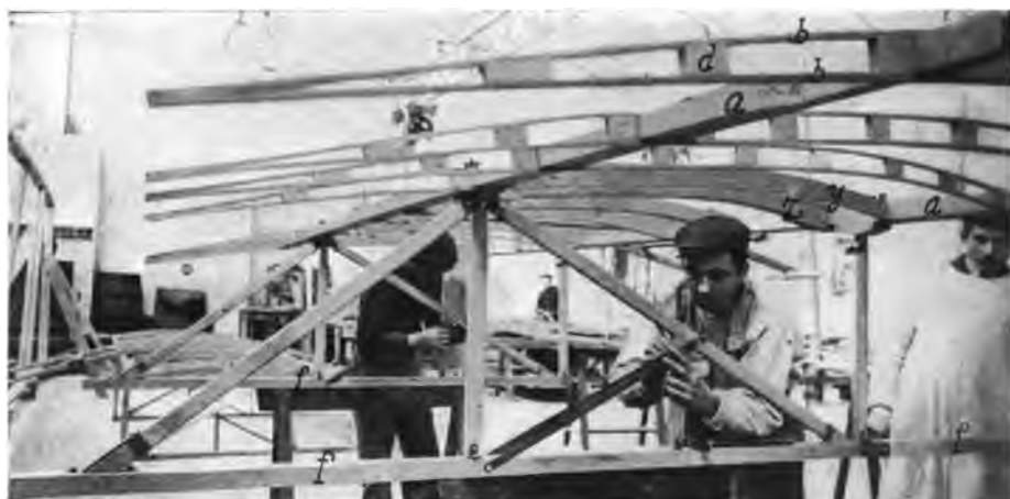
FIGURE 194.—Side View of Wright Runner Construction. The reference lettering is the same as in the preceding.
