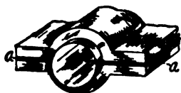
FIGURE 155.—Adjustment of Plain Bearing. To tighten the bearing one or more of the thin liners of sheet metal at a a are removed.
