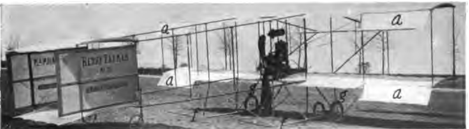
FIGURE 81.—Alleron Control of Farman Biplane. The four hinged allerons are shown at aaaa .
