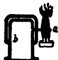
FIGURE 124.—Hot-Tube Ignition. Compression of a portion of the charge in the cylinder b into the tube through the lamp c occasions combustion of the fuel.
