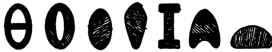
FIGURE 178.—Sections of Wooden Spars. The ends sought in these different constructions are light weight, great strength, and a minimum resistance to passage through the air.
