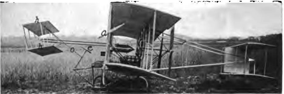
FIGURE 80.—Side View of Pischoff & Koecklin Biplane, showing one of the allerons very clearly at a . The ingenious system of controlling the forward elevator hh by direct connection of the steering rod e to the steering pillar o is of interest.
