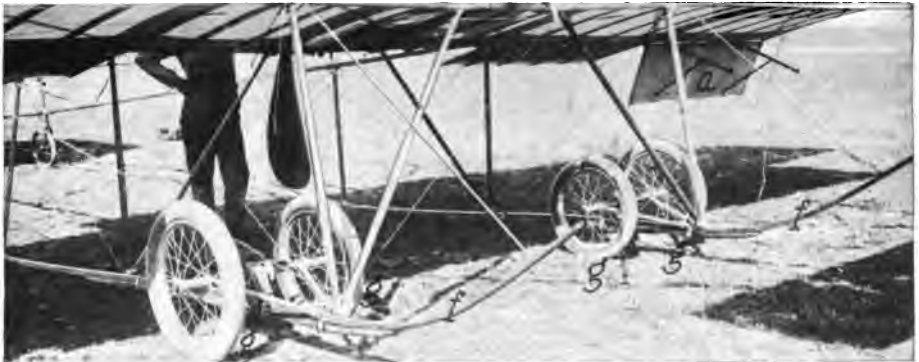
FIGURE 174.—Alighting Gear of Farman Machine. Note the runners f f and the wheels g g .
